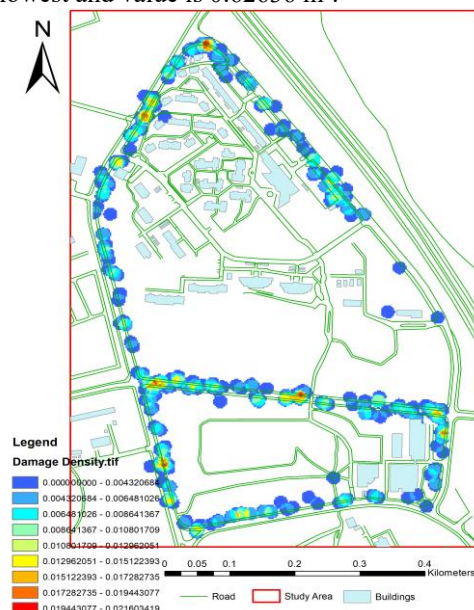
Figure 04: Damage density of the sidewalk
