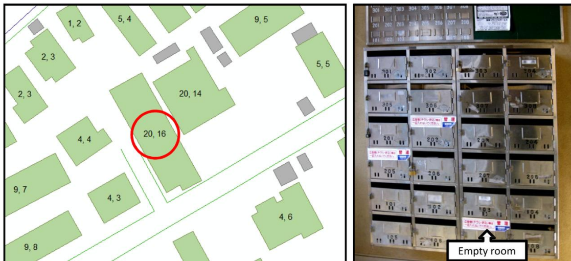
Figure 3-15: Result validation by Single Multiple Unit mail-box usage condition Left value is estimated from Floor approach and right value is estimated from LIDAR approach, actual building population is 21
